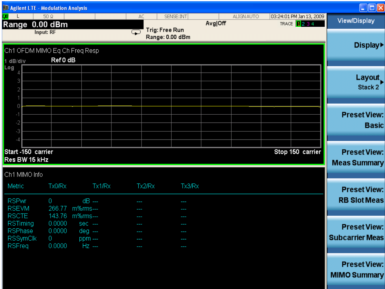
Figure 3-12 Modulation Analysis Measurement Result - MIMO Summary Preset View
